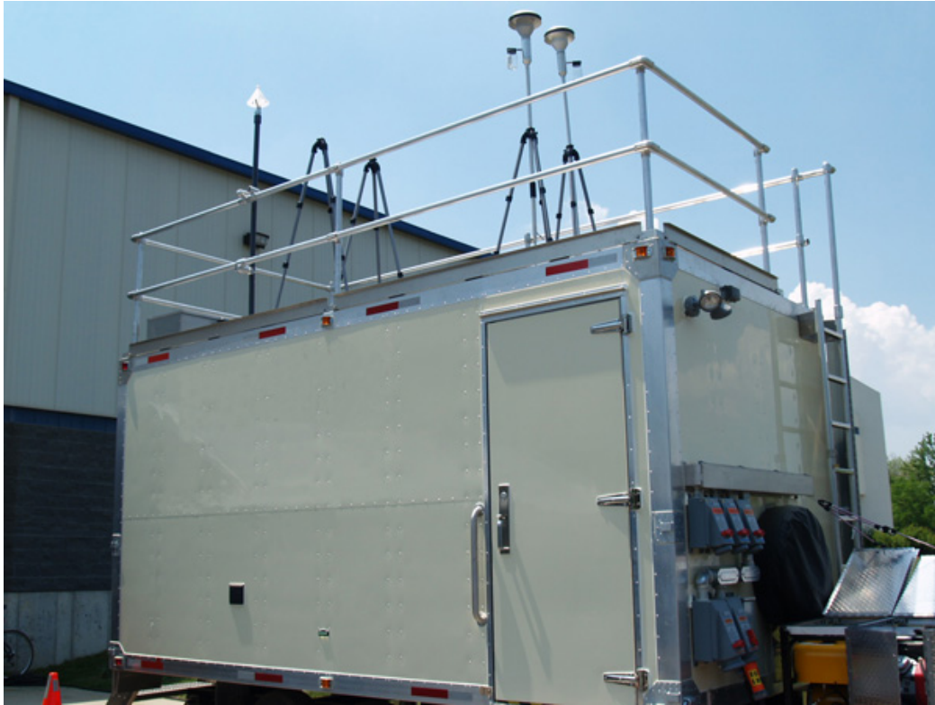
FIGURE 3 EXAMPLE OF AN AIR QUALITY MONITORING SHELTER
